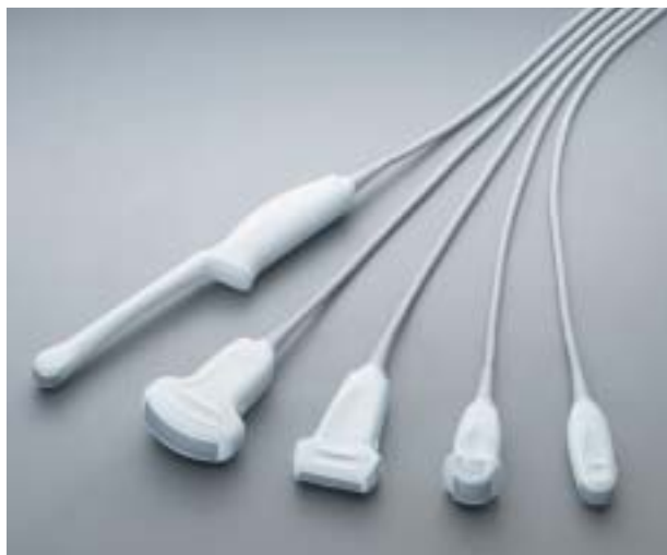
FIGURE 1: High-resolution transducers operate at 2–10 MHz for the following applications (left to right): intracavitary; abdominal; breast, superficial, and vascular; transthoracic and trauma; and vascular access. Photograph courtesy of SonoSite, Inc.
